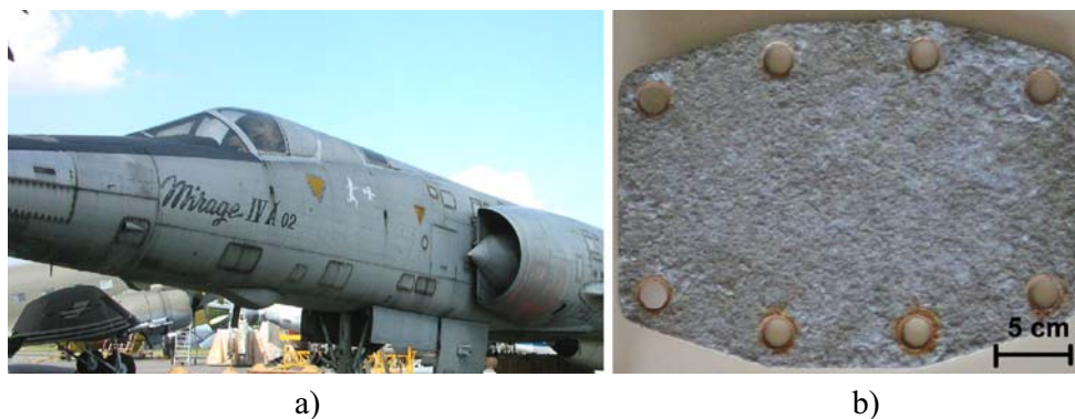
Fig. 1 a Mirage IV in the Air and Space Museum, Le Bourget, France, b macroscopic aspect of the inspection hatch under the wing of the plane (exterior face)
