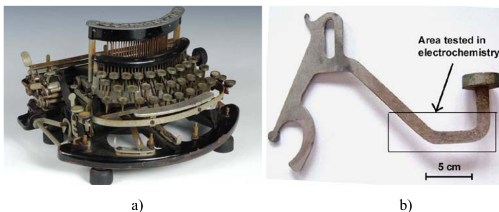
Fig. 9 a Typewriter TYPO model no. 1 of Manufrance (1913–1923), b a key in nickel-plated steel of the typewriter used for the electrochemical measurements
